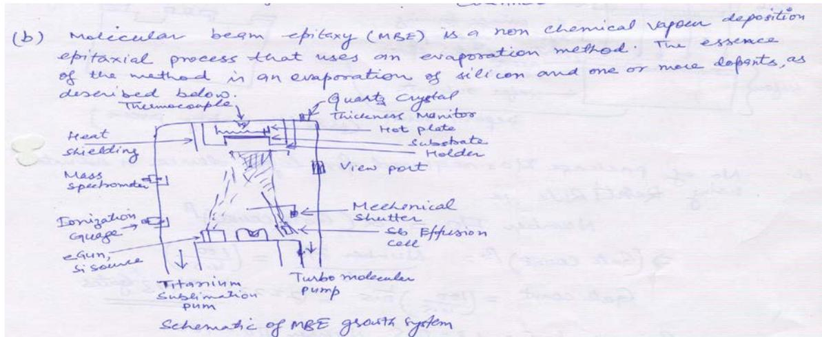
The evaporated species are transported at a relatively high velocity in vacuum to the substrate. The relative low vapour pressure of Si and the dopant ensures consideration at low temperature substrate. The Silicon MBE is performed under <sup>ultra</sup>high vacuum conditions of  $10^{-8}$  to  $10^{-10}$  torr. The mean free path of atoms is
